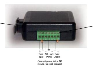
Removable edge connector Insert a small screwdriver in the upper slot to force open the wire clamp. Push all the way in to open fully. Place stripped wire end(s) in the open clamp and withdraw screwdriver.
